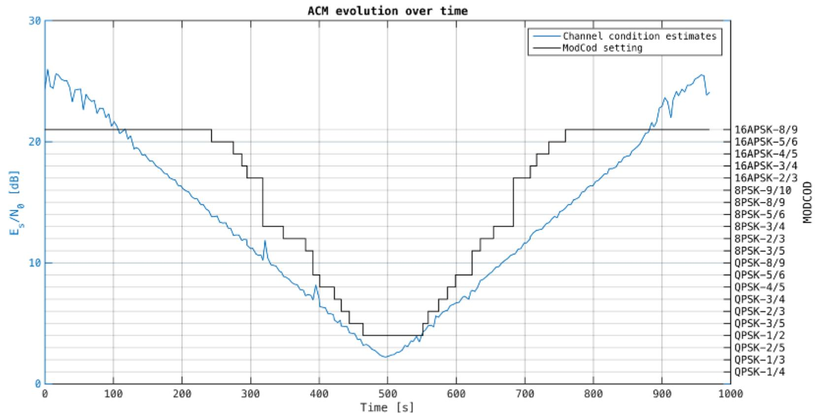
ACM adapts modulation and coding depending on link conditions to achieve QEF target
