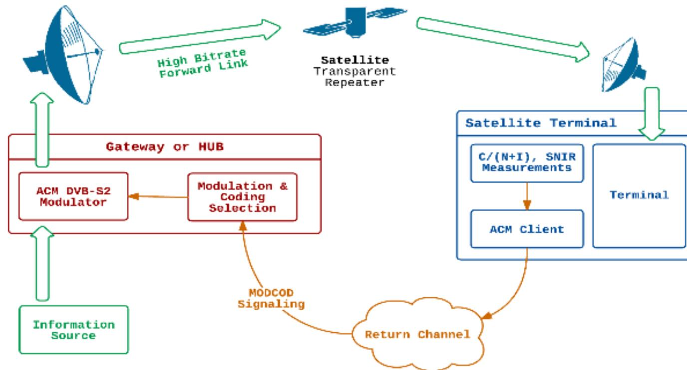
→ Complex system as we need to have a **return channel** , a **reliable estimation of CNIR** and an **ACM client/controller**
