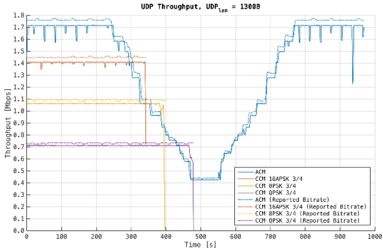
Naturally, UDP throughput varies as modcod parameters vary. UDP throughput disappears quickly because of LDPC BER curve steepness.
